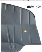
These floor plates are for the reparation of T2 from 08/'67-07/'71, which can be used in the front compartment. They are an imitation, but they have all the ridges like the originals. Sold by piece and we've already some in stock.
