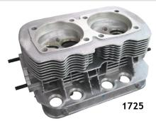
These '041' cylinder heads are since a long time for sale on the market. Due to the increasing demand we have taken them in our program. They are the same heads as BBT #1720 (1600cc) only larger valves stick into (intake 40mm i.o. 35.50mm / exhaust 35.50mm i.o. 32.00mm) with the '041' cylinder head, which gives of course a gain of power. We have opted to sell the cylinder heads bare, so that the customer can decide which parts he needs for his motor. Sold per piece and stock already available.
