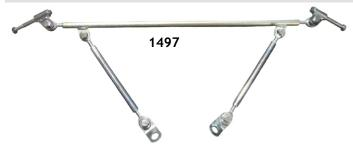
This set makes that the body won't crack when leaving, in case we've assembled a high power engine. This simple assembly system can be used on all beetles and KG without too many adjustments, welding or boring like the other kits for sale. The materials used are of high quality and galvanized for a long use and maintenance. These rods can be assembled between the shock absorber supports and the gear box supports on the body. Sold per piece and already some in stock.
